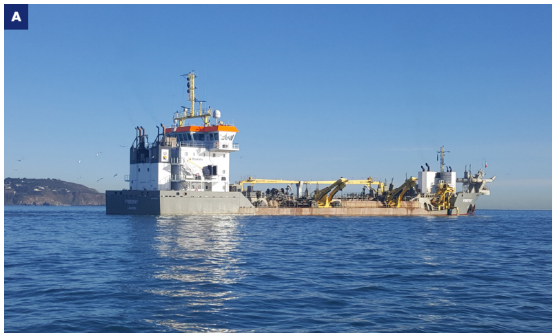
The project was carried out using the trailing suction hopper dredger Freeway, supported by the survey launch Smit Neyland and the plough vessel Norma.
