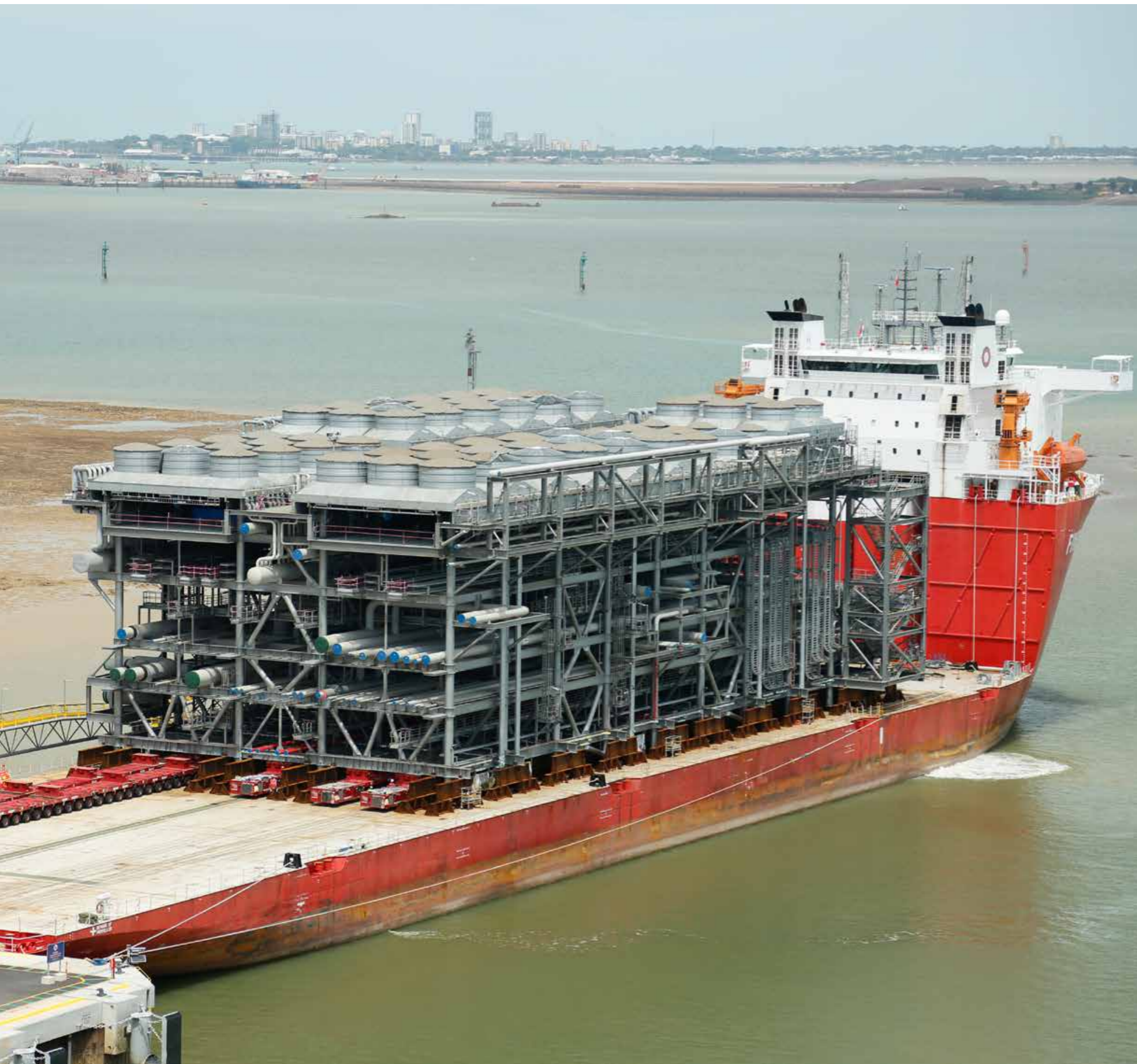
Darwin, Australia LNG project, including 19 transports of modules with Finesse from different fabrication yards to the LNG plant in Darwin
