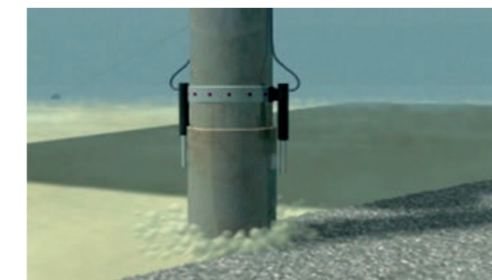
The Scradeway® method produces a smooth rock bed, reducing the costs of the tunnel structure.
